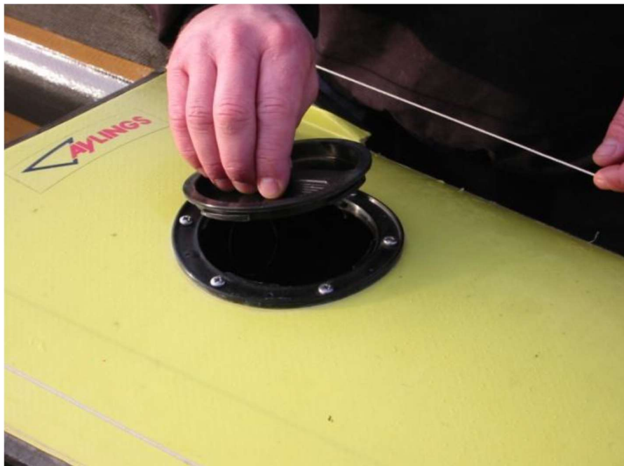
Fig 1: Fitting buoyancy hatch.
