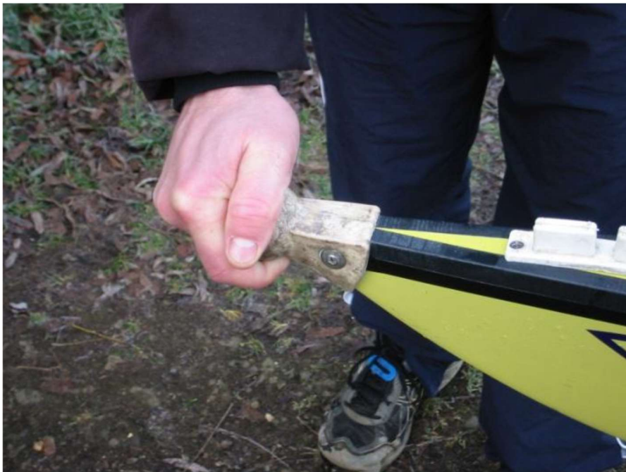
Fig 2: Checking the bow ball is secure.
