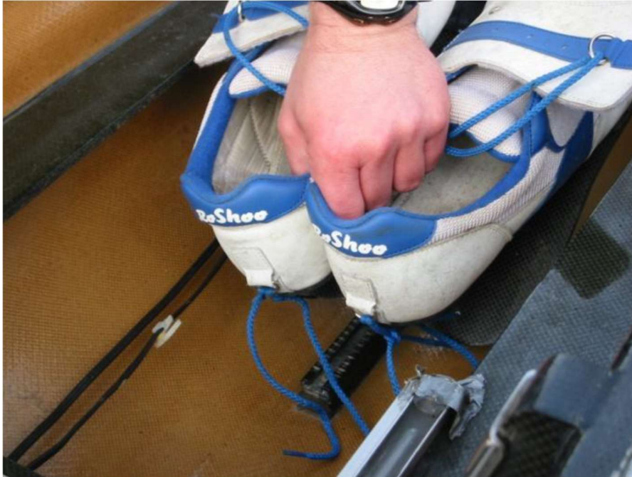
Fig 3: Checking that the heel restraints are connected.
